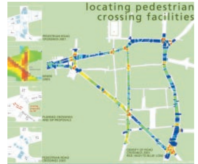
Left: To support traffic reform proposals in Shoreditch, London, Intelligent Space Partnership carried out surveys of pedestrian crossing behaviour which highlighted potentially dangerous informal crossing points. Alteration to the placement of crossing facilities meant that new facilities were located where pedestrians wanted to use them
