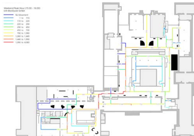
Proposed Modelled Flow during the Peak Hour (15:00-16:00) during a Blockbuster Exhibition
